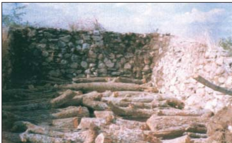
Figure 2.5: Firewood logs in a Traditional Lime Kiln (Lirangwe, Blantyre) Source: MIRTDC, Blantyre
